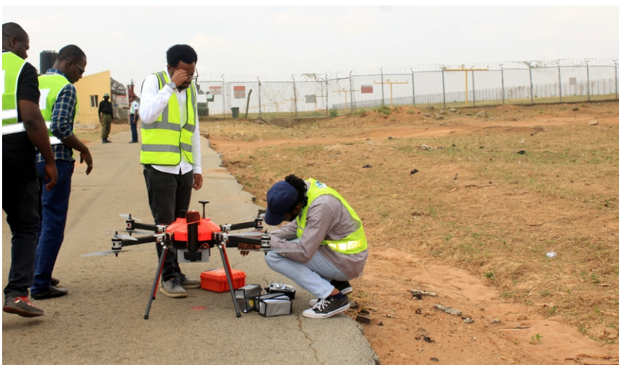
Prepping the Colibrex COL-X8 flight calibration drone for flight inspections demonstration at the Abuja International Airport on 27 March, 2025.
